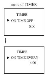
1.2.3. Pressing the () button set the TV into standby mode. At the preset time the TV will automatically turn on to preset channel. To cancel ON TIME, set ON TIME OFF.
